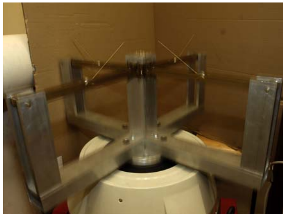
Figure 6. Experimental implementation of the parametrically excited pendula of Figure 3(c).
