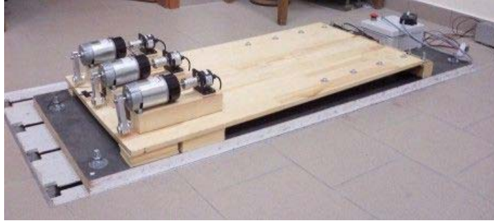
Figure 4. The experimental rig: three direct-current electrical motors mounted on the wooden plate which can oscillate vertically.
